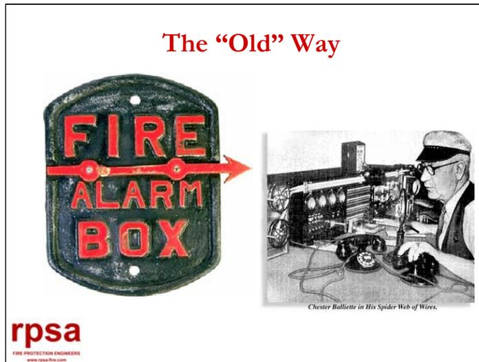
It was not uncommon in the early 20th century to have initiating devices (thermostats, sprinkler waterflow switches and manual boxes) connected to a circuit that directly controlled bells connected in the fire house. One property, one bell. In another configuration, an automatic coded telegraph transmitter might be used on a city or privately owned telegraph circuit.
